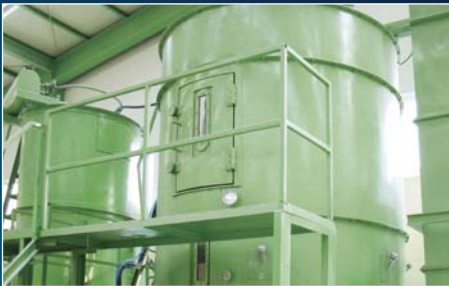
2. Dryer • Air dryer • Removal of the moisture from the raw materials
