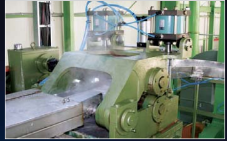
6. Crimping Part • Crimping system with steam and punch function
