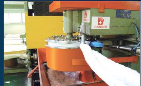
8. Cutting Part • Cutting the crimped tow • 32mm - 102mm
