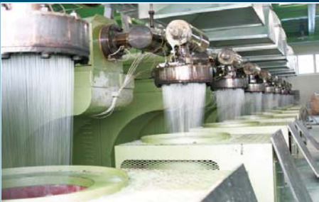
3. Extruder • Spinning extruder through dried raw materials • To prevent deformation by 22°C cooling system
