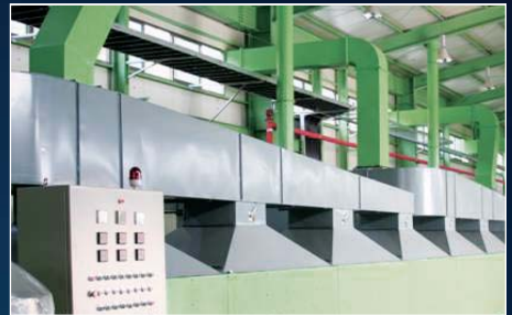
7. Tenter • Drying moisture of stretched fiber • preventing loose crimp
