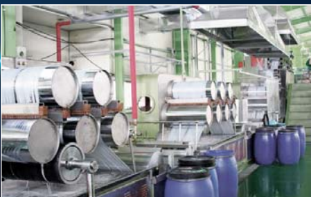
5. Stretching Part • Three-times progress of stretch fiber
